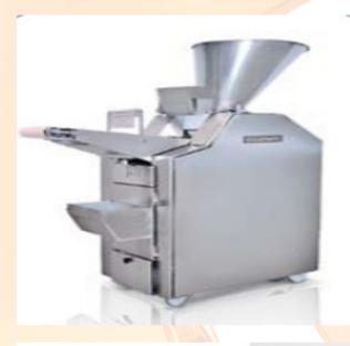
DIVOBAR weighs the dough loaded to its hopper by means of its own weight & vacuum generated by the piston movement across cylinder; and cuts the dough in the required weight without damaging it by rotation movement.
