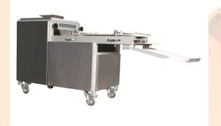
MOLDOBAR Long Moulding Machine is used for molding of dough coming from intermediate prover.
