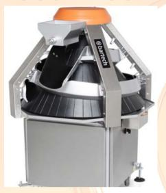
RONDOBAR Dough rounding machine rolls the dough coming from dividing machine, by means of clockwise rotating Teflonised aluminum conical and Teflon coated aluminum tracks
