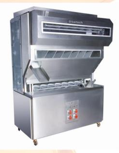
BARTECH Intermediate Proving machine proves dough coming from dough rounding machine for a while and then transfers them to the molding machine or to another place for different operation. This is the first proving step for dough coming from dough rounding machine.
